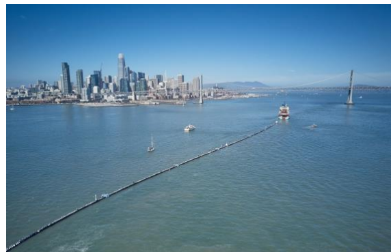
This technology is powered by wind and wave energy which allows it to concentrate plastic debris towards the center of the system.
